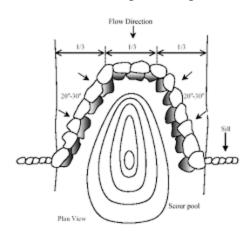
crosses a barrier perpendicular to the barrier. Consequently, they direct water away from the stream banks and direct it down the middle of the channel to the gage as shown in the schematic and in the accompanying photo of the new weir at the Harrison Bridge gage.
